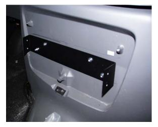
**4.** Mark and drill four 5/32" diameter holes and attach floor mount plate with # 10 x 1" sheet metal screws. Also add two  $\frac{1}{4}$ " x  $\frac{3}{4}$ " carriage bolts facing up.
